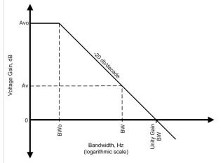
"BWo" is the cutoff frequency built into the device by the manufacturers.
