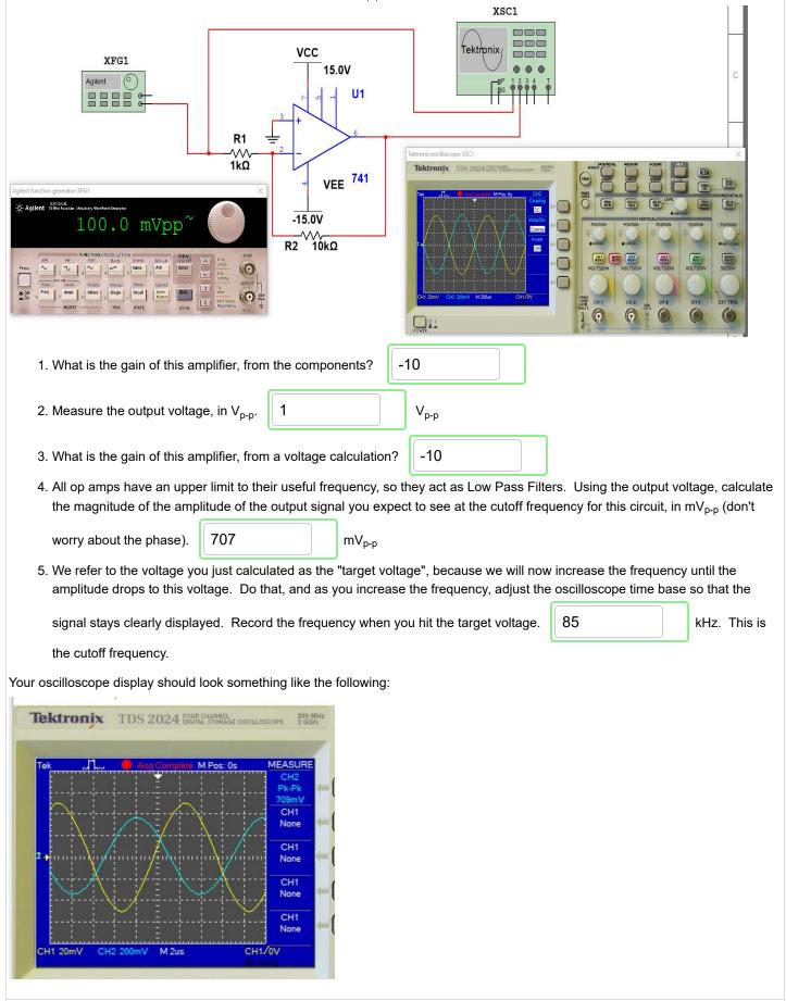
Notice two things: First, the amplitude has dropped as closely as I can get it to the target voltage of 707 mV<sub>p-p</sub>. Second, the output signal is no longer just "inverted" -- it now lags by another 45° from where it started. If we kept going, at very high frequencies it would lag by a full 90° for a single capacitor (that's from the "-j" in all of the frequency-related math that you've done in other courses).
